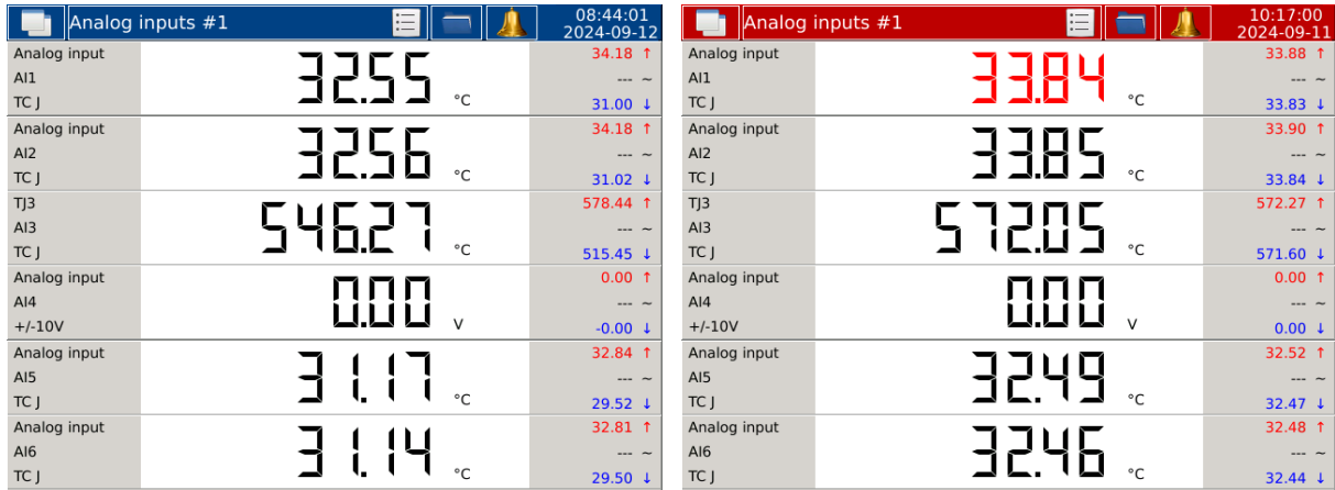
Figure 86: Screen view without active alarm. Figure 87: Screen view with active alarm.
